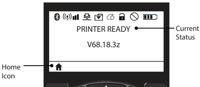
Figure 16: Idle Display Screen (QLn420 and QLn Healthcare)
