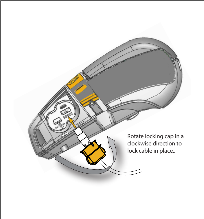
Figure 23: Communications Port Strain Relief (QLn420 Shown)
