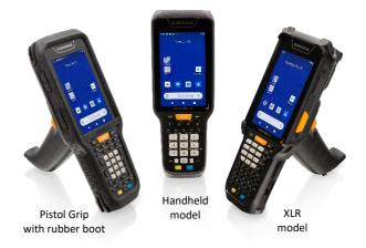
Packed with the latest technology, the Skorpio X5 is equipped with the largest high visibility 4.3" display in its class, providing plenty of space for the most modern applications. It is powered by the market leader Qualcomm Snapdragon® 660 platform running at 2.2 GHz, the latest Google OS Android™ 10 with Google Mobile Services (GMS) and it is validated by Google as an 'Android Enterprise Recommended' (AER) rugged device.
