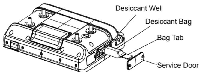
7. Carefully place the service door onto the right side of the housing.
