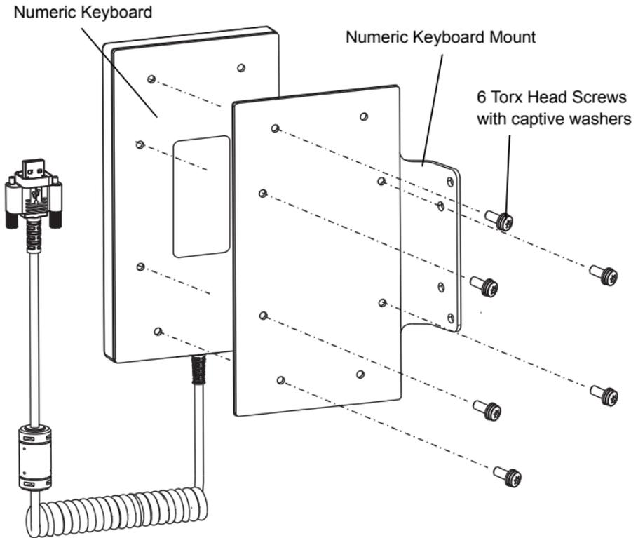
3. Attach the numeric keyboard mount to the VC70, using four M5x14mm Torx head screws with captive washers. Tighten the screws.
