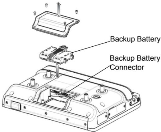
6. Connect the Backup Battery connector to the connector inside the Backup Battery well.
