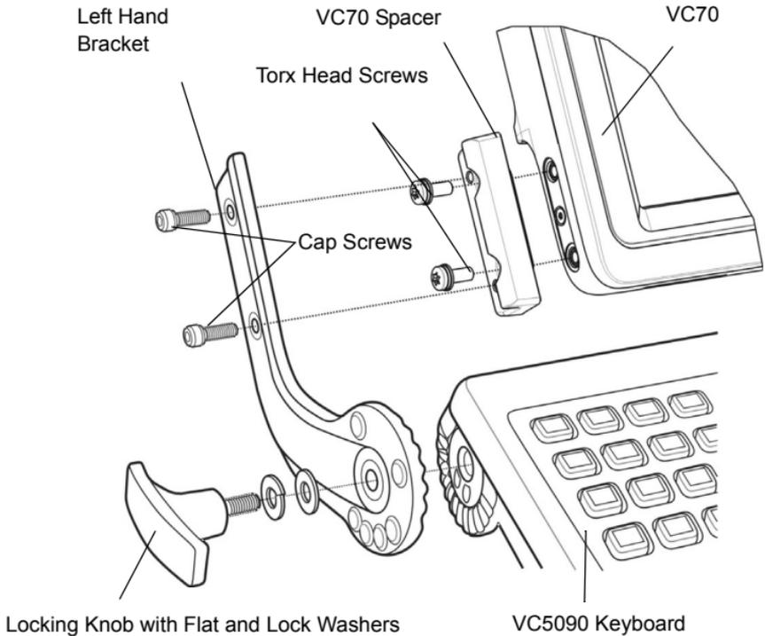
2. Attach the VC5090 keyboard brackets (part of the VC5090 keyboard assembly) to both sides of the VC70, using the cap screws with captive washers. Only tighten the cap screws three turns.
