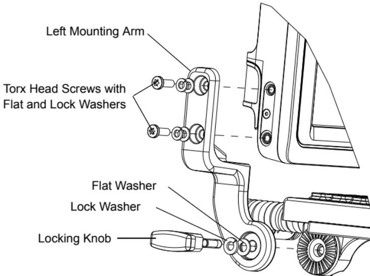
3. Insert the keyboard locking knobs through the washers and brackets and screw into the keyboard tray. Tighten fully to lock into place.
