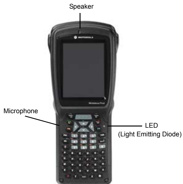
Figure 1-1 Front View of the Workabout Pro4 7528 Long Alphanumeric Keyboard
