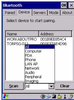
This menu allows you to limit the scope of the scan to a particular type of device. If, for example, you choose *Computer* from this menu, only computers within range of the WORKABOUT PRO<sup>3</sup> are listed in the *Device* tab. Choosing *All* lists all detected devices.
