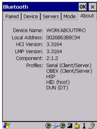
*Device Name* displays the broadcasted name of the WORKABOUT PRO<sup>3</sup>. The name can be changed in the *System Properties* applet – *Start>Settings>Control Panel>System icon>Device Name tab*.
