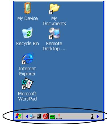
The WORKABOUT PRO<sup>3</sup> is equipped with a taskbar at the bottom of the screen. It displays icons through which you can view the battery capacity and radio signal quality of your unit. If the hand-held is attached to a charger, cradle or docking station, an associated icon is displayed. In addition, the taskbar displays the application(s) currently running on your unit and the security level assigned to your WORKABOUT PRO<sup>3</sup>.
