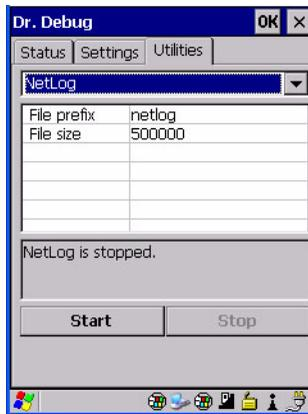
The *Utilities* tab is used to log network traffic. When you tap on the *Start* button, debug data is collected so that, if necessary, it can be forwarded to a Psion Teklogix technician for evaluation.
