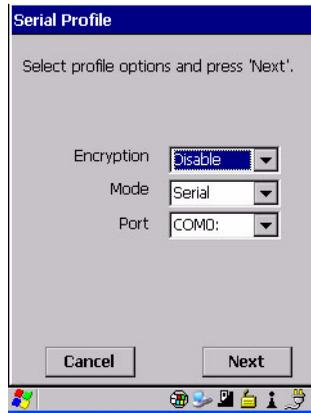
This dialog box offers a number of additional options such as enabling *Encryption* and selecting three different *modes*: *Serial*, *ActiveSync* and *Scanner*
