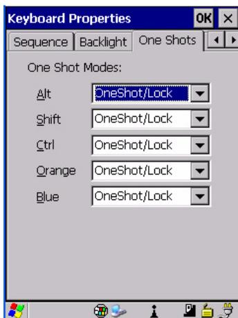
The options in this tab allow you to determine how modifier keys on your WORKABOUT PRO<sup>3</sup> behave. For each modifier key – [ALT], [SHIFT], [CTRL], [ORANGE] and [BLUE] – you have the following options in the drop-down menu: *Lock*, *OneShot*, and *OneShot/Lock*.
