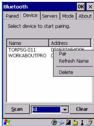
The *Device* pop-up menu allows you to pair a device, update a device name or delete a device from the list.
