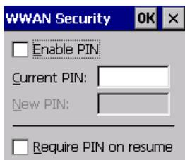
The *Security Configuration* dialog box is accessed through the *Tools* menu. The *Security Configuration* dialog box allows you to enable, disable and change the PIN. You will need the current PIN to make any of these changes. The PIN must be enabled in order to be changed. (If the PIN is disabled, the *New PIN* entry field is greyed out.)
