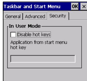
If you check *Disable hot keys*, the *Application from Start menu hot key* field becomes enabled. Use this field to enter the name of the application you want to run when the user presses the *Menu* hot key – *[FN/BLUE] [0]*.
