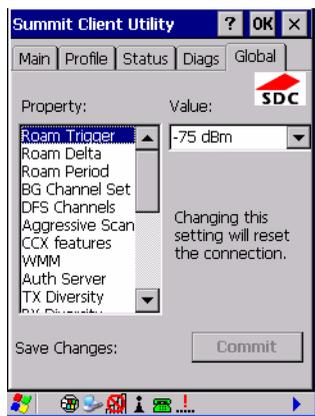
The *Global Settings* tab allows you to define radio and security settings that apply to all profiles, along with settings that apply specifically to the SCU.
