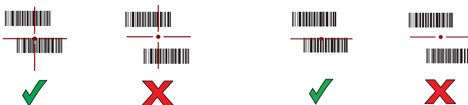
Figure 39 Pick List Mode with Multiple Barcodes in Aiming Pattern: Standard and Extended Range
