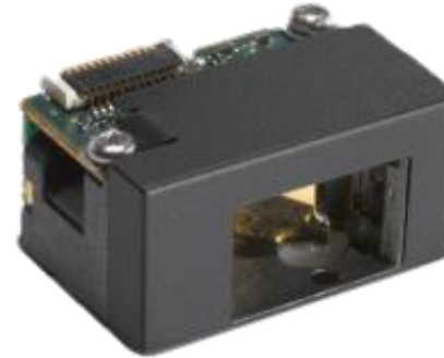
MC92N0-GA SE965 1D Standard Range Laser
