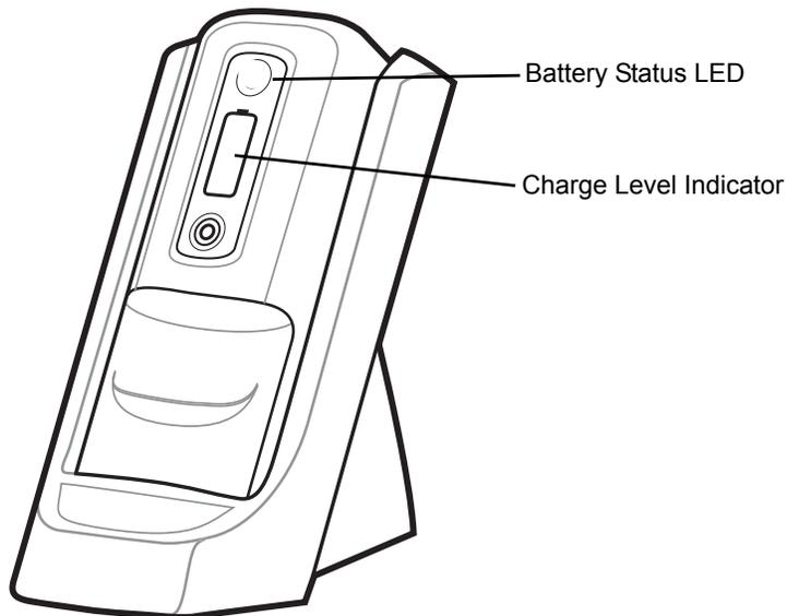
**Figure 2-6** Battery in Single Slot Battery Charger
