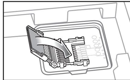
**Figure 1-4** Insert microSD Card in Holder
