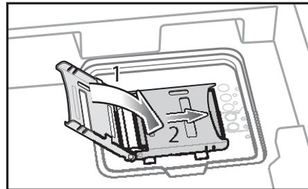
**Figure 1-7** Insert microSD Card in Holder
