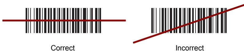
**Figure 4-2** Linear Scanner Aiming Pattern
