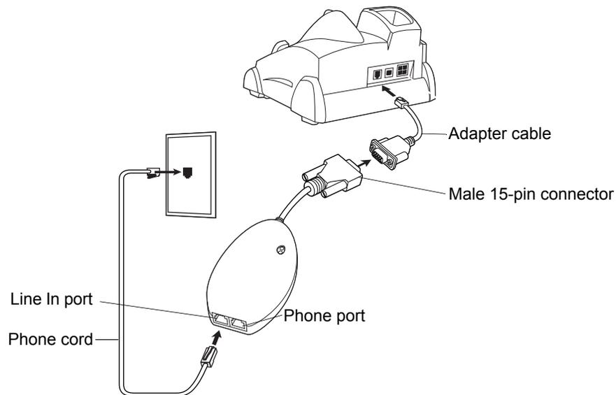
**Figure 5-19** Modem Module Connection - Single Slot Serial/USB Cradle
