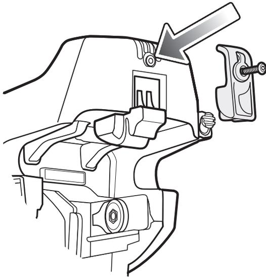
Figure 5-23 Locking Mechanism
