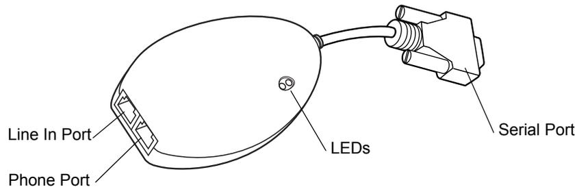
**Figure 5-17** Modem Dongle
