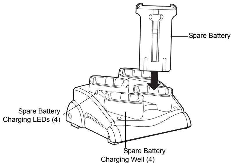
**Figure 5-5** Four Slot Spare Battery Charger
