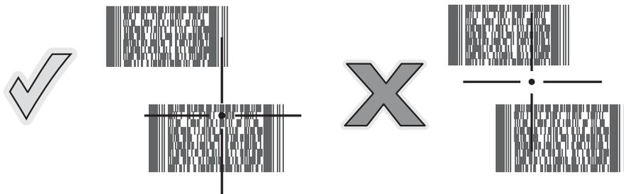
**Figure 3-4** Standard Range Pick List Mode with Multiple Bar Codes
