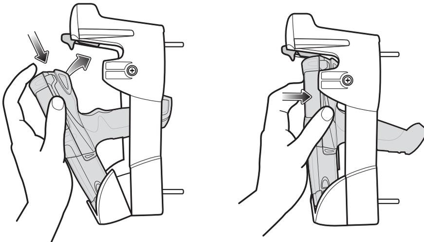
Figure 5-21 Insert MC9190-G into Forklift Cradle
