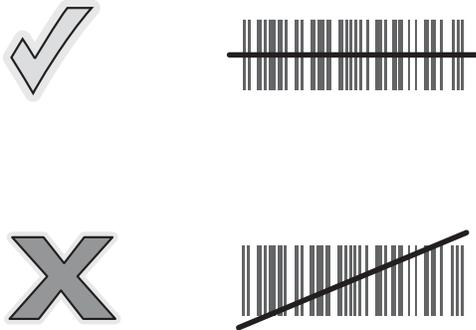
**Figure 3-1** Laser Aiming
