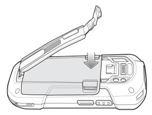
6 Place hand strap clip into hand strap mounting slot and pull down until it snaps into place.
