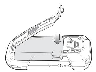
13 Place hand strap clip into hand strap mounting slot and pull down until it snaps into place.
