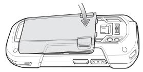
3 Press the battery down into the battery compartment until the battery release latches snap into place.
