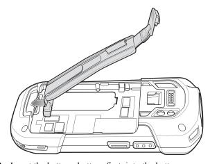
3 Insert the battery, bottom first, into the battery compartment in the back of the TC70.
