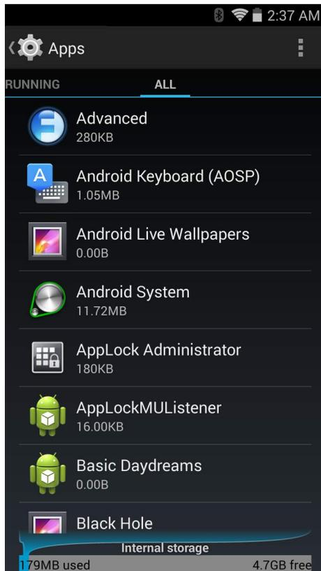
The **Manage Applications** screen has four tabs, with lists of applications and their components in each. At the bottom of each tab is a graph of the memory used by the items in the list and amount of free memory.
