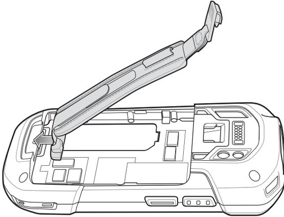
**10** Insert the battery, bottom first, into the battery compartment in the back of the TC70.
