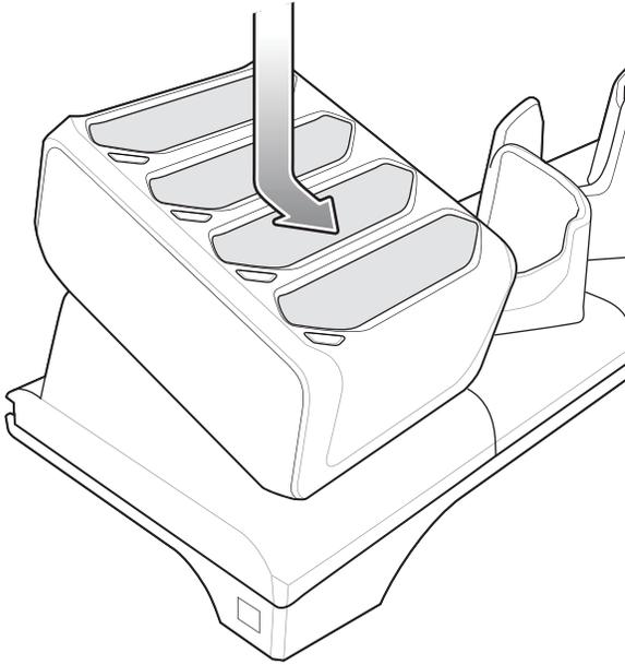
**10** Slide the Four Slot battery Charger down toward the front of the cradle.
