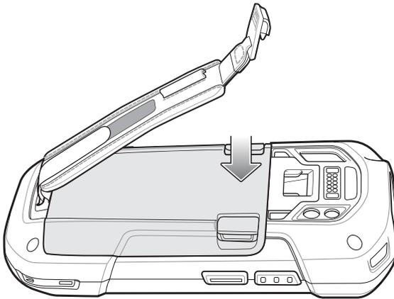
**13** Place hand strap clip into hand strap mounting slot and pull down until it snaps into place.
