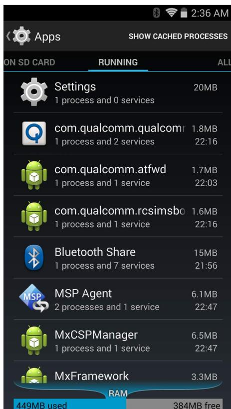
The bar at the bottom of the screen displays the amount of used and free RAM.
