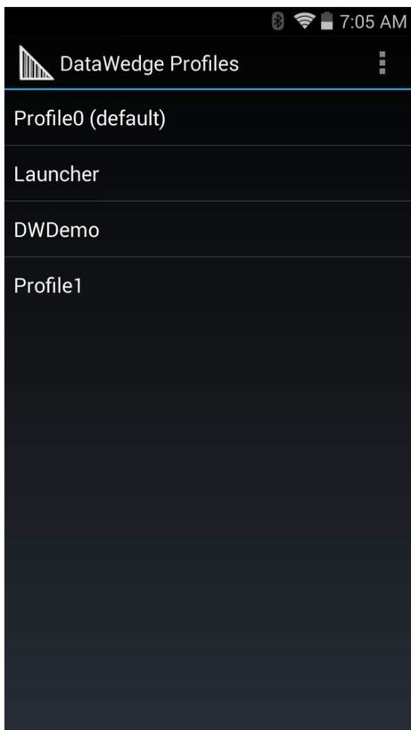
Profile names are color coded. Enabled profiles are white and disabled profiles are gray.
