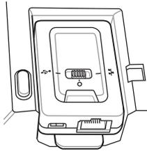
For Ethernet communication, slide the switch to the
