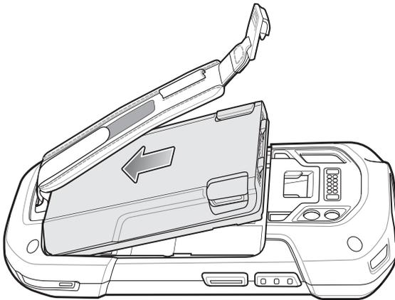
**11** Rotate the top of the battery into the battery compartment.
