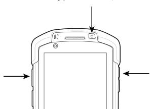
Figure 1-15 Three Button Reset
