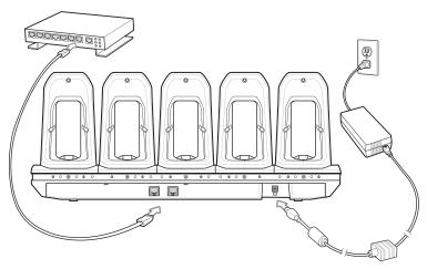
Figure 2-28 5-Slot Ethernet Cradle Setup
