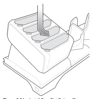
Figure 2-24 Install Four Slot Battery Charger
