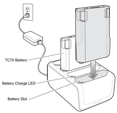
Figure 2-45 Four Slot Battery Charger
