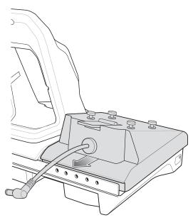
Figure 2-39 Install Adapter
