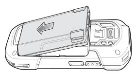
Figure 1-7 Insert Bottom of Battery into Battery Compartment
