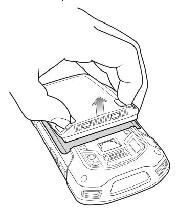
Figure 2-48 Lift the Battery
