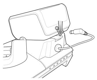
Figure 2-26 Press Release Latch
