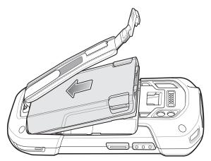
Figure 1-4 Insert Bottom of Battery into Battery Compartment
