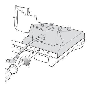
Figure 2-23 Secure adapter to Cradle
