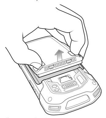
Figure 1-11 Lift the Battery
