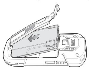
Figure 2-50 Insert Bottom of Battery into Battery Compartment
