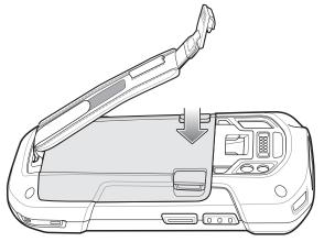
Figure 2-51 Press Down on Battery
