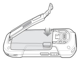
Figure 1-5 Press Down on Battery
