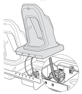
Figure 2-37 Disconnect Cup Cables
