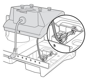
Figure 2-21 Connect Adapter Power Cable
