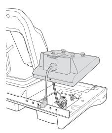
Figure 2-38 Connect Adapter Power Cable
