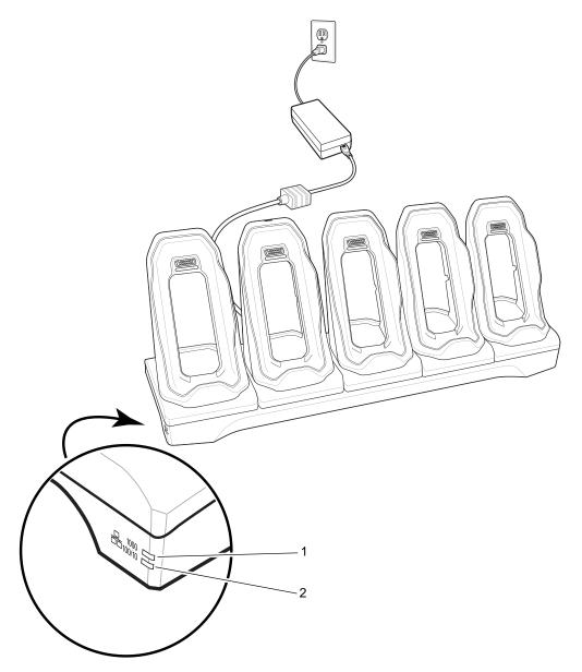
Figure 2-27 5-Slot Ethernet Cradle
