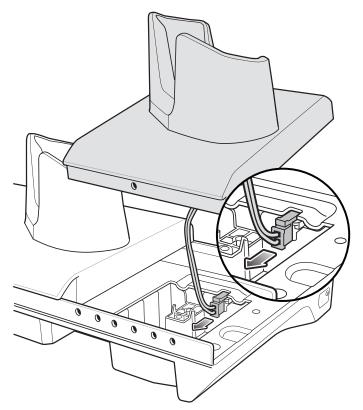
Figure 2-20 Disconnect Cup Power Cable
