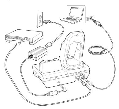
Figure 2-6 2-Slot USB/Ethernet Cradle
