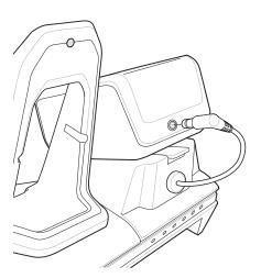
Figure 2-42 Connect Adapter Power Cable
