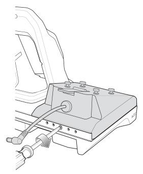
Figure 2-40 Secure adapter to Cradle
