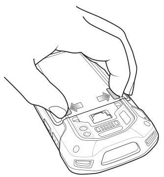
Figure 2-47 Press Battery Latches
