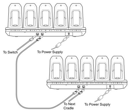
Figure 2-29 Daisy-chaining 5-Slot Ethernet Cradles
