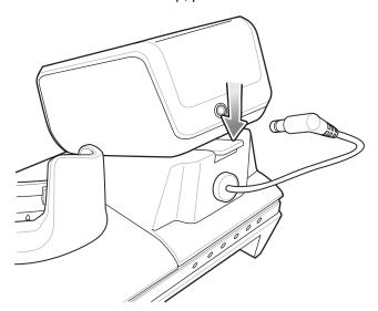
Figure 2-43 Press Release Latch
