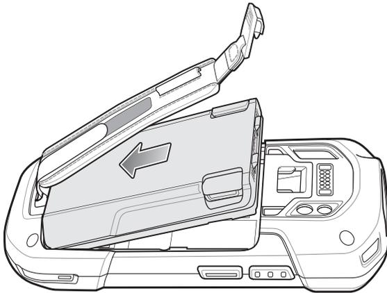
**Figure 2-50** *Insert Bottom of Battery into Battery Compartment*
