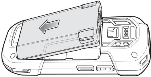
**Figure 1-7** *Insert Bottom of Battery into Battery Compartment*
