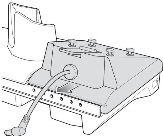
**Figure 2-22** *Install Adapter*
