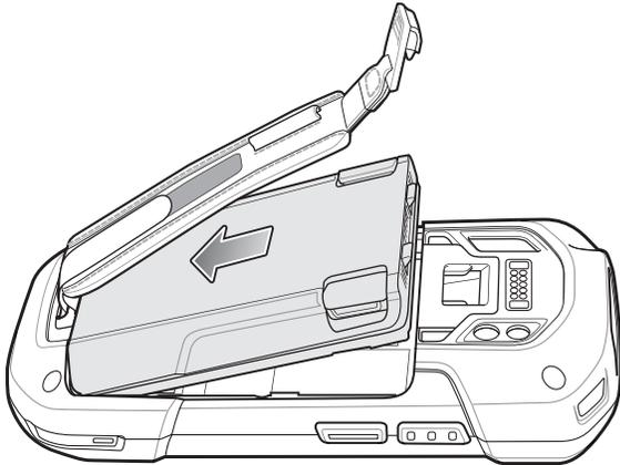
**Figure 1-4** *Insert Bottom of Battery into Battery Compartment*
