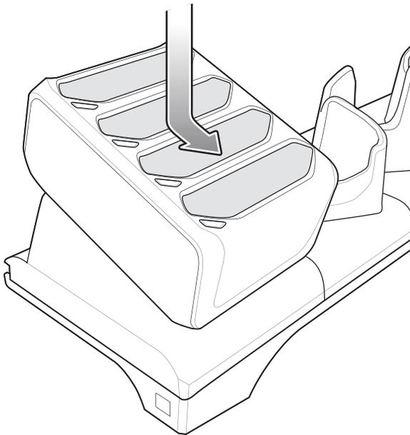
**Figure 2-24** *Install Four Slot Battery Charger*
