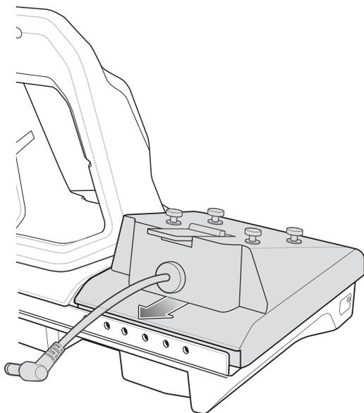
**Figure 2-39** *Install Adapter*
