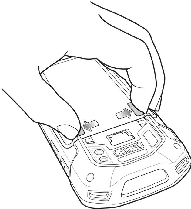
**Figure 1-10** *Press Battery Latches*
