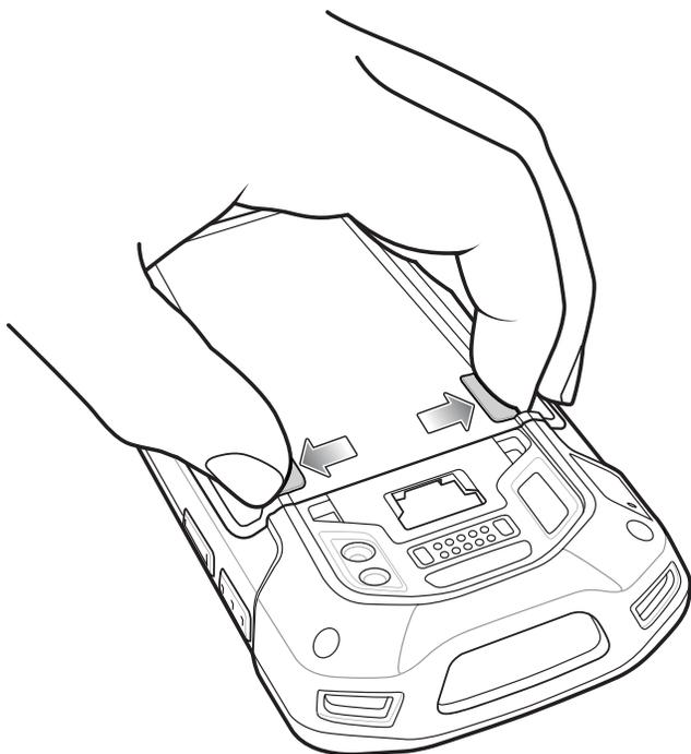
**Figure 2-47** *Press Battery Latches*
