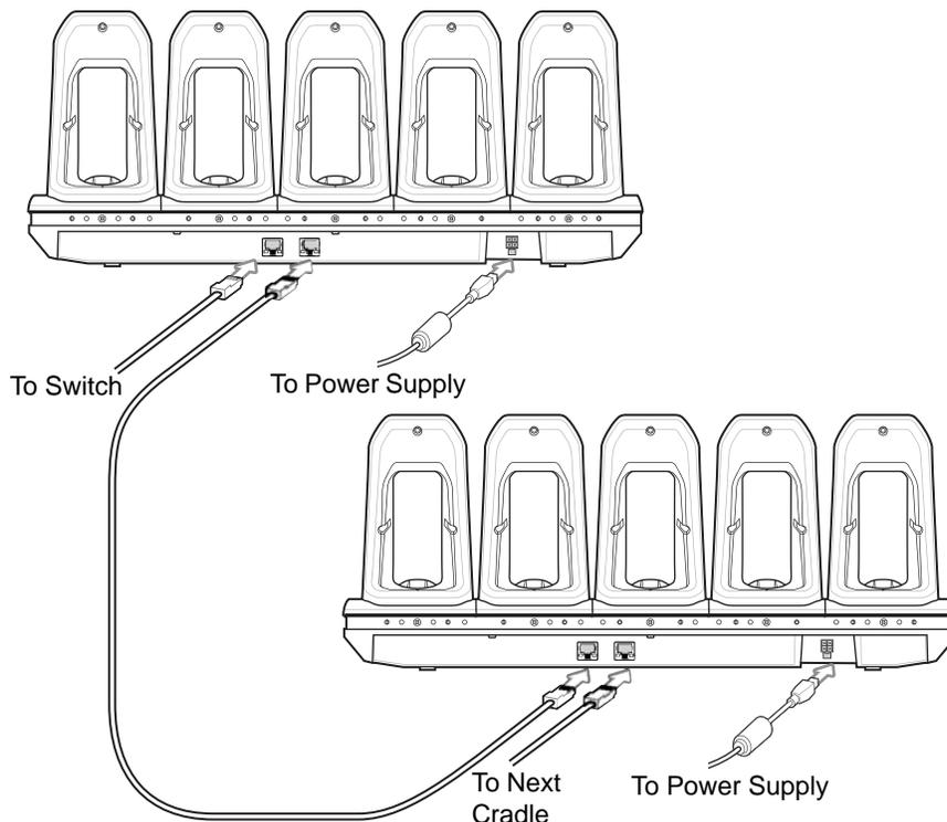
**Figure 2-29** *Daisy-chaining 5-Slot Ethernet Cradles*
