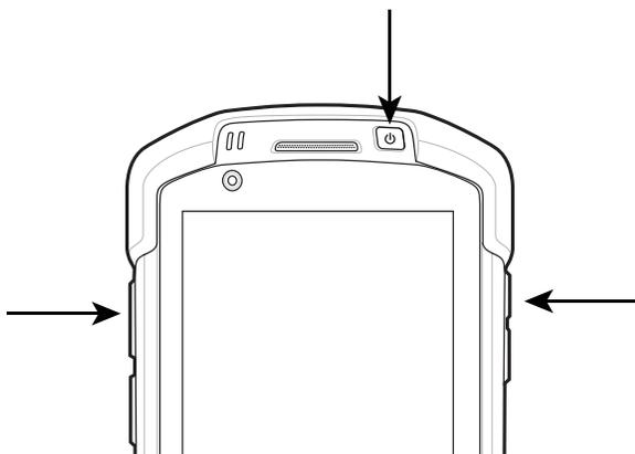
**Figure 1-15** *Three Button Reset*
