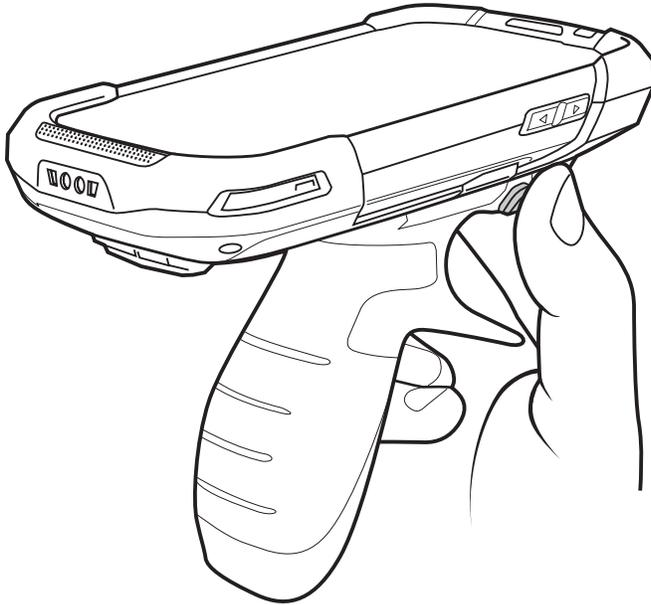
**Figure 6-51** *Press Release Latches*
