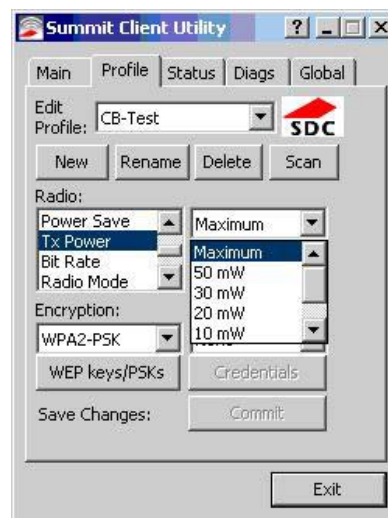
Figure 2-2 Configuring the antenna transmitting power with SCU (example)
