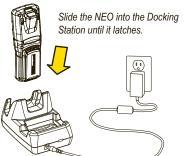
Note: Use only the universal AC power supply approved by Psion Teklogix for use with the Docking Station.
