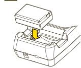
Note: During charge, the LED indicator on the NEO is YELLOW until charging reaches 75%.
