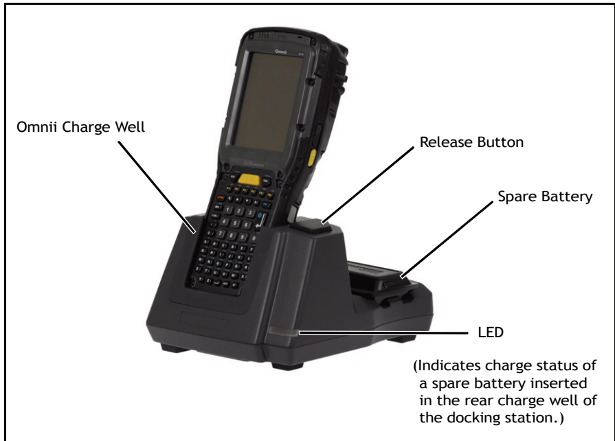
Figure 6.8 Desktop Docking Station - Models ST4002 and ST4003
