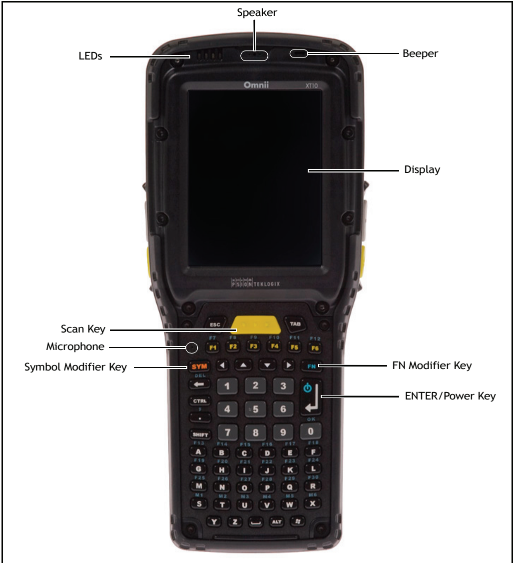
Figure 2.1 Front View of Omnii XT10 Model with Alphanumeric Keyboard
