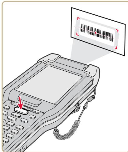
For near or close-in scanning distances of 30 cm (11.8 in) or less, use the laser pointer as a guide and aim slightly to the right of the center of the bar code. Make sure the illumination beam covers the bar code you are trying to decode.
