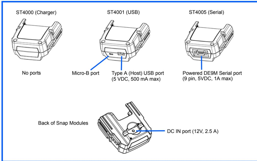
Figure 5-6 Snap Module Installation
