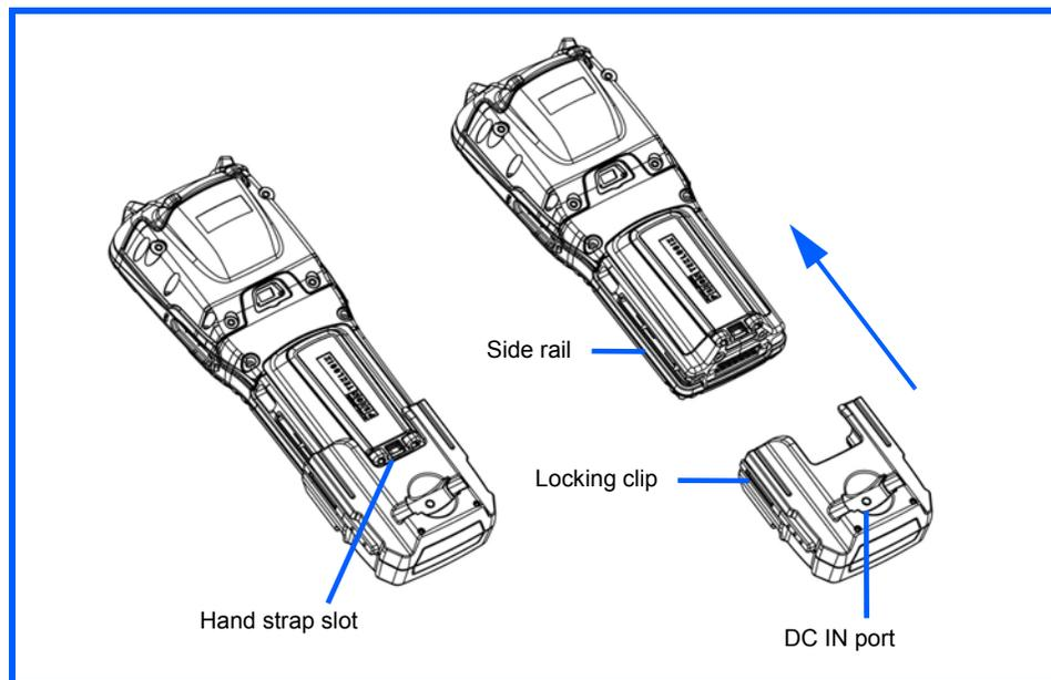
To attach the Snap Module charger to Omnii:
