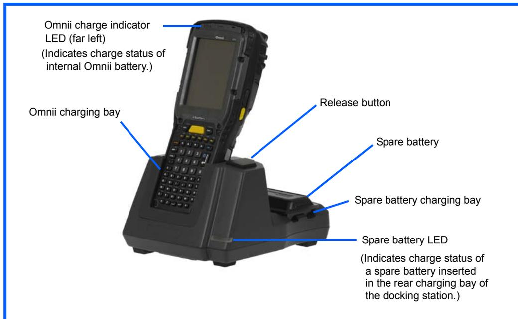
The desktop docking station storage temperature is -30°C to +60°C (-22°F to 140°F). Operating temperature and humidity are: 5 - 95% non-condensing and 0°C to 40°C (32°F to 104°F).
