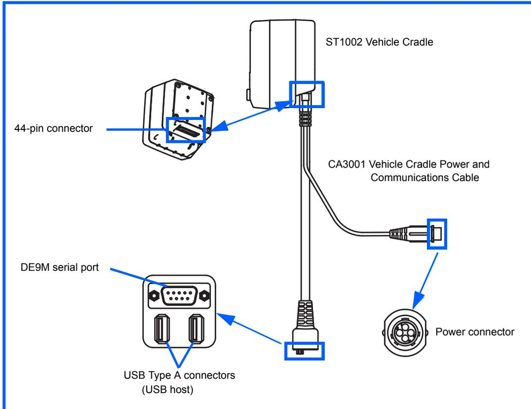
The following are the pin assignments of the interfaces.
