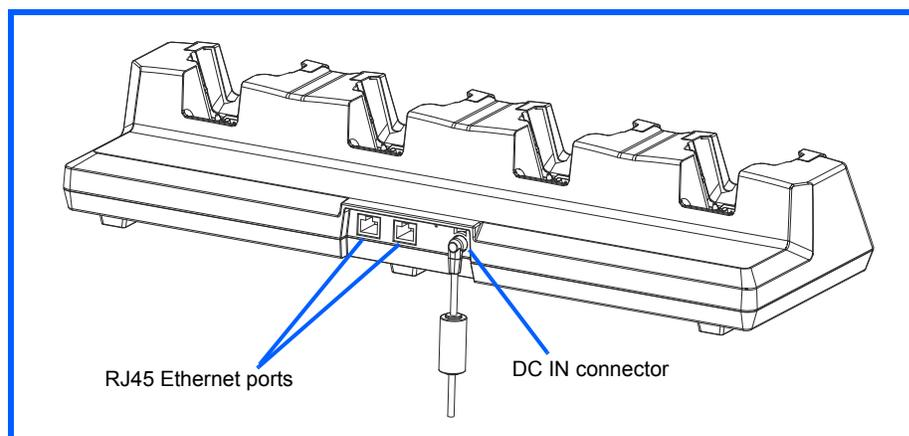
The ST4004 Quad Docking Station is designed to accept up to four Omnii hand-held computers. The docking station powers the units and their internal battery charger. The docking station also connects up to four of the hand-held computers to a 10/100 Base-T Ethernet network and allows for Ethernet data transfer. An additional Ethernet interface is available for connecting more docking stations downstream, up to 4 on the same network.
