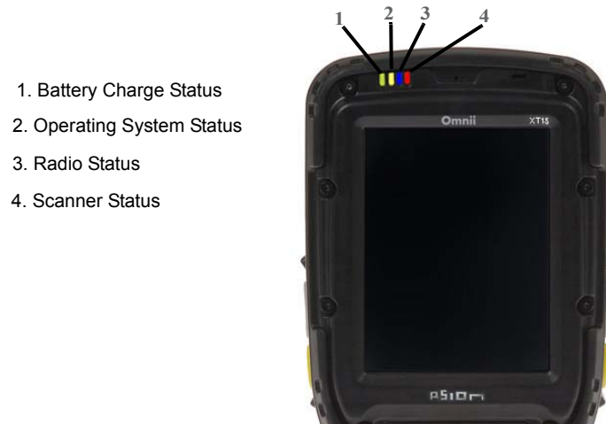
Figure 2-3 LED Status Indicators
