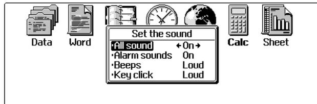
A dialog line is usually unavailable because of the setting on another line in the dialog. For example, select 'Sound' on the 'Control' menu in the System screen. If you set the 'All sound' line to 'Off', the bullets will disappear from the start of the other dialog lines and you cannot change their settings.
