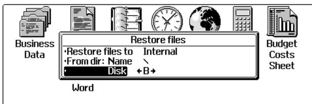
2. Set the 'Restore files to' line to the disk you want to use for the restored files, usually the Internal disk.
