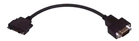
Cable from device (Handylink) to male DB9 RS232. Straight through cable, Power on Pin 9 (5V @ 500mA). Connects to printers, scanners, or most other peripherals. 15cm straight cable
